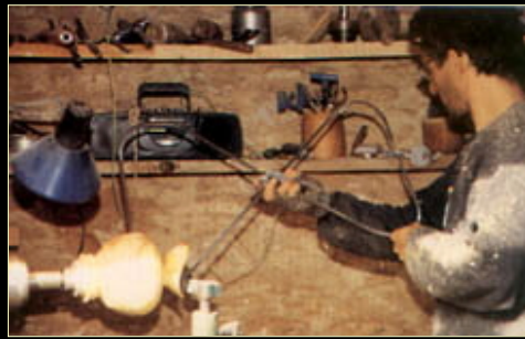
Occasionally, Alain checks thickness with huge, homemade callipers.
